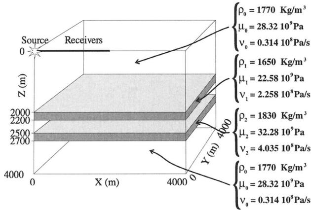
FIG. 3. Two thin attenuating layers are embedded in a homogeneous background medium. The parameters of each layer are plotted on the right. Equivalently,  $c_0 = 4000 \text{ m/s}$ ,  $c_1 = 3700 \text{ m/s}$ , and  $c_2 = 4200 \text{ m/s}$ ;  $Q_0 = \omega\mu_0/\nu_0$ ,  $Q_1 = \omega\mu_1/\nu_1$ , and  $Q_2 = \omega\mu_2/\nu_2$ .
