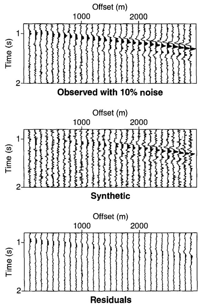
FIG. 7. Noisy synthetic seismograms, corrupted by Gaussian noise band limited to the same frequency as the data, are used as the observed data (top panel). The offsets correspond to 29 receiver locations. The middle panel shows the synthetic seismograms obtained by Ray-Born approximation for the recovered model. On the bottom, residuals have a small amplitude, which proves the convergence of the procedure.
