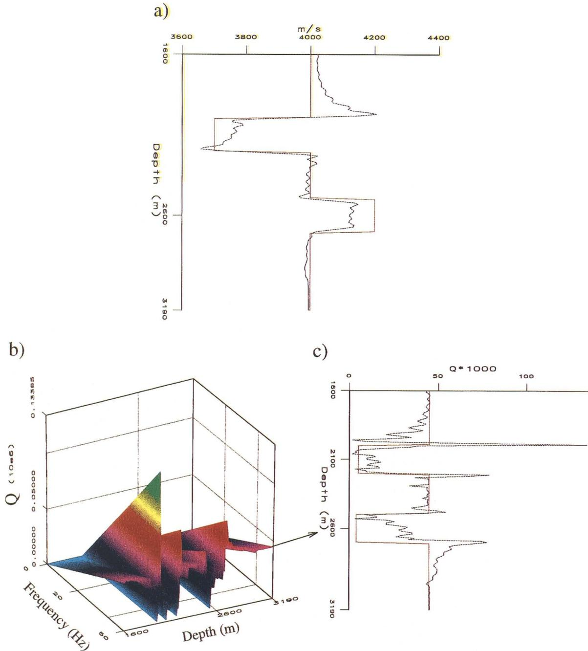
FIG. 5. Recovered medium shown as profiles of the global velocity in (a), and the global quality factor in (c). In (b), the recovered quality factor is plotted for each frequency. The block diagram explicitly shows the linear frequency dependence of the considered  $Q$  factor. In (c), the true model is superimposed with the recovered profile at 50 Hz. The continuous line (red) is the true model, the dotted line (black) is the recovered model.
