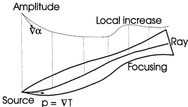
FIG. 1. Ray tracing for an attenuating medium requires supplementary parameters compared to the elastic case, i.e., the vector  $\nabla\alpha$  in the direction of maximum spatial attenuation.
