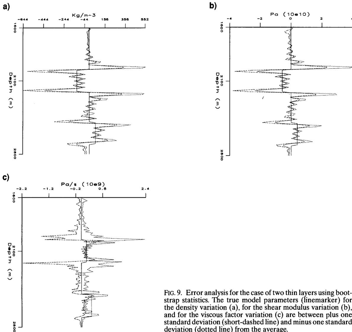
FIG. 9. Error analysis for the case of two thin layers using bootstrap statistics. The true model parameters (linemarkers) for the density variation (a), for the shear modulus variation (b), and for the viscous factor variation (c) are between plus one standard deviation (short-dashed line) and minus one standard deviation (dotted line) from the average.
