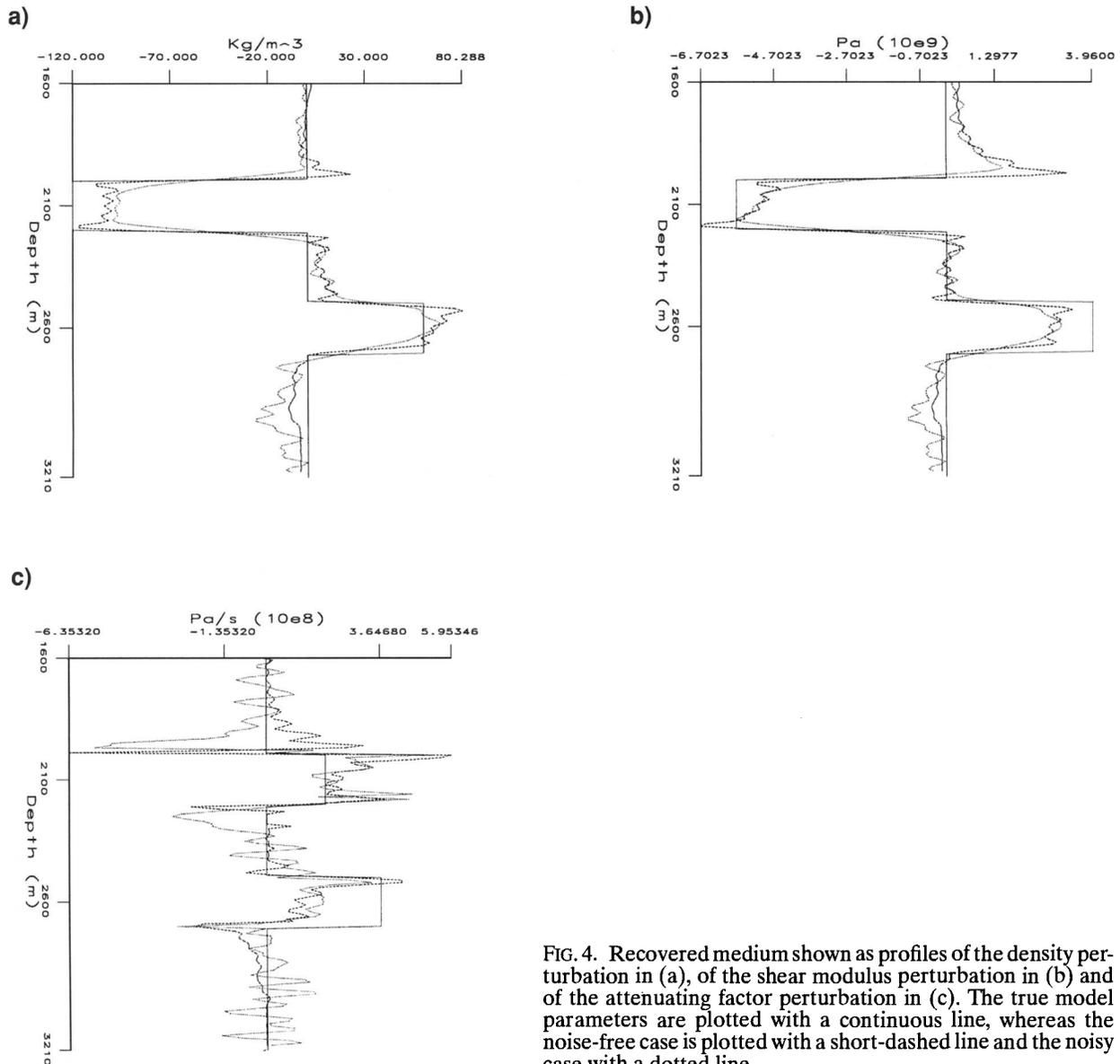
FIG. 4. Recovered medium shown as profiles of the density perturbation in (a), of the shear modulus perturbation in (b) and of the attenuating factor perturbation in (c). The true model parameters are plotted with a continuous line, whereas the noise-free case is plotted with a short-dashed line and the noisy case with a dotted line.
